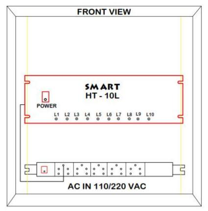
**SMART** HOTLINE PA TELEPHONE SYSTEM has two DESKTOP HOTLINE PA TELEPHONES connected by single pair wire with one **SMART CONTROLLER UNIT**, the controller is AC powered (220/110 V AC).
